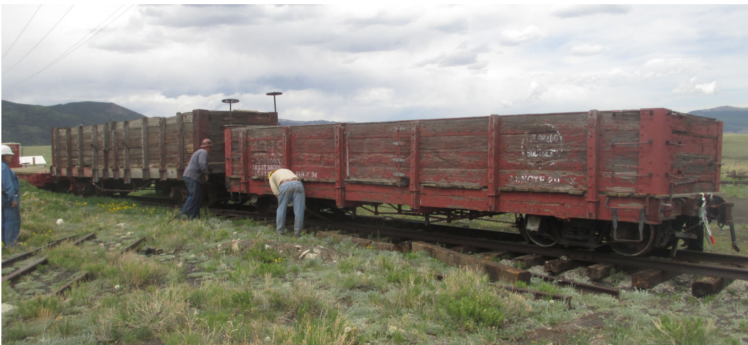
Figure 1. The differences between the common Denver & Rio Grande Railroad “High Side” gondolas and the Colorado & Southern Railway gondolas can be clearly seen in this photo showing the D&RG car on the left. (Photo from South Park Rail Society, June 2018. Photo by Tim Bain)
