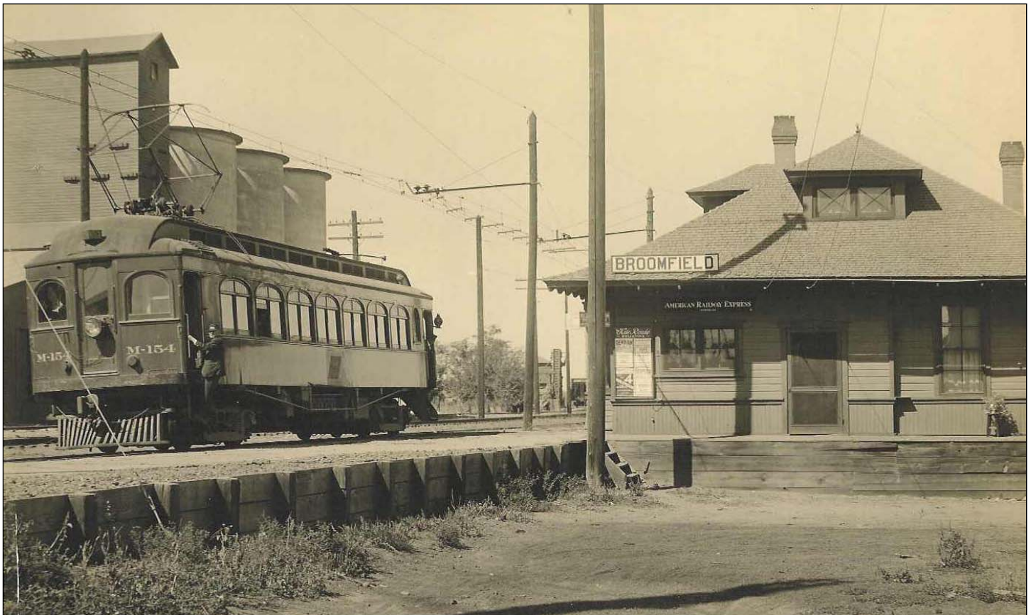
Figure 10. Denver & Interurban motorcar M-154 is shown in this 1912 of the Broomfield Depot. The diamond-shaped pantograph is mounted atop the car making contact with the overhead catenary which carried the electrical power. Courtesy of Broomfield Depot Museum, photographic collection.
