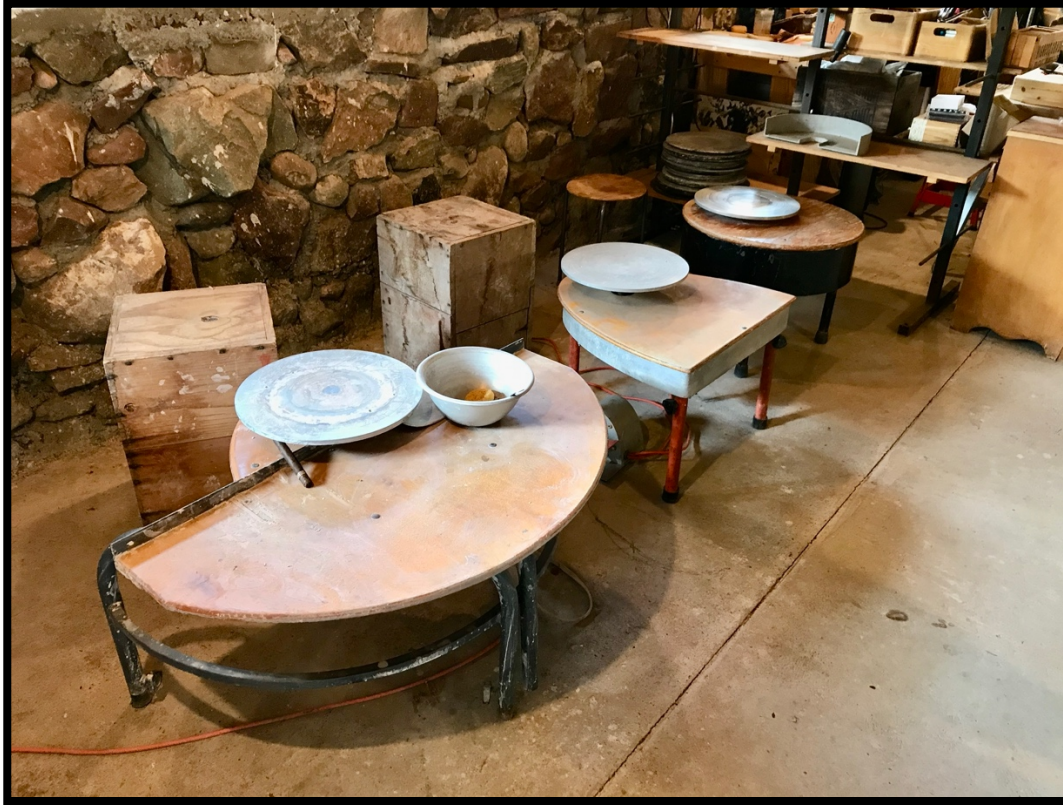
Photo 34: Studio Building Interior, Soldner Patented Electric Kickwheels.
