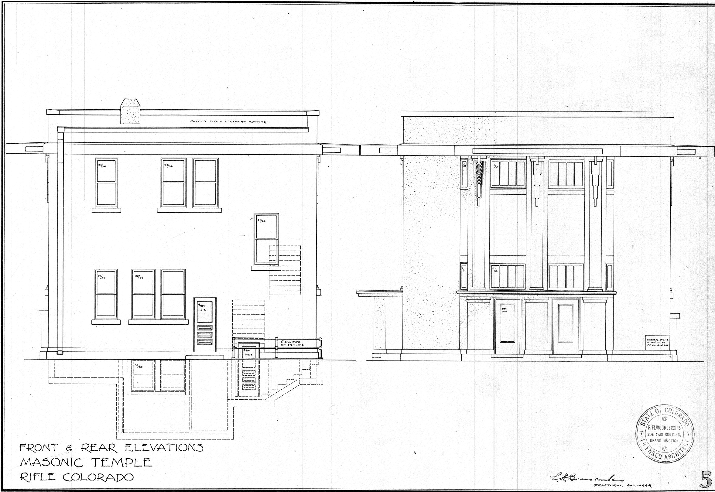
Fig. 4. West and East Elevations Notice front porch at east is not full-width.
